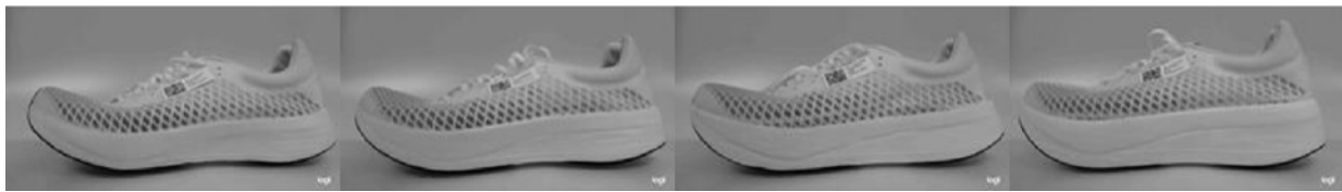
Figure 0.1: The four footwear conditions tested (left – right, 35-, 40-, 45-, and 50-mm).
