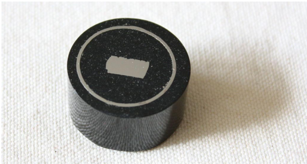
Figure 4-3 Mounted Metallurgical Sample of SCC Affected Pipeline, 32 mm Diameter
