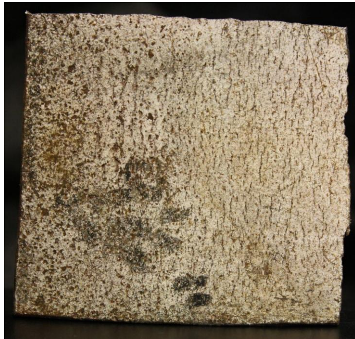
Figure 2-3 Field Pipeline Sample with SCC Colony Oriented Up/Down on Right Hand Side
