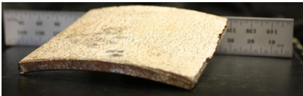
Figure 10-1 Pipe Specimen Showing Radial Curvature and Surface Cracks
