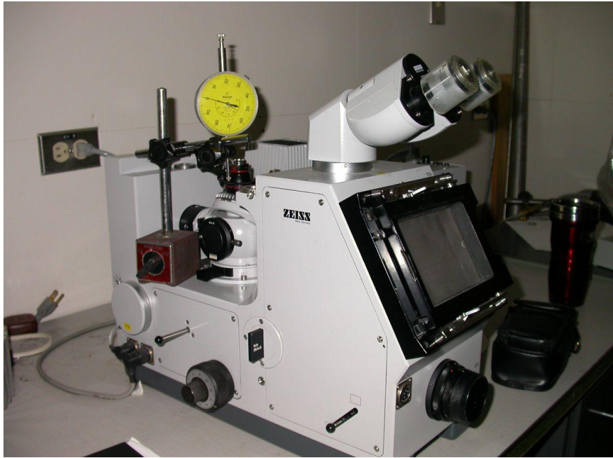
Figure 10-5 Experimental Setup for Calibrating Lens Movement to the Adjustment Gauge
