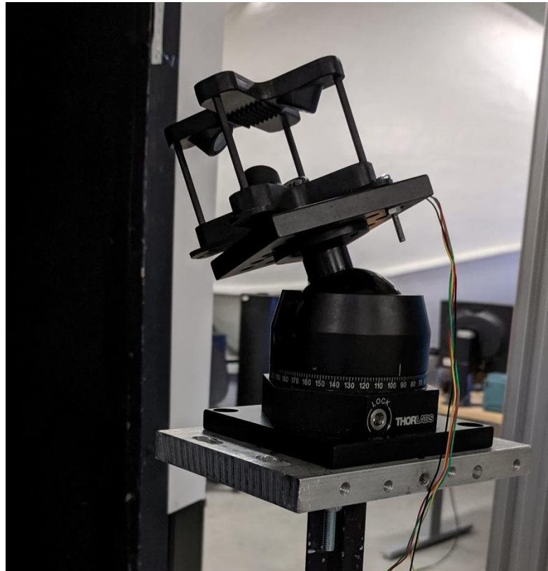
Figure 3.4: TSM attached to the ball mount during testing. The TSM was positioned so the sensor was slightly overhanging the leading edge of the mounting plate.
