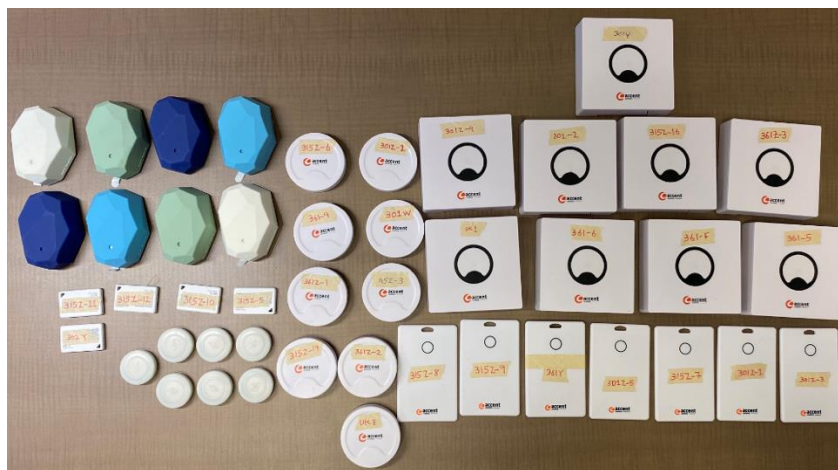
Figure 2.10. Six different types of BLE beacons from three different BLE manufacturers used in real-world experiment
