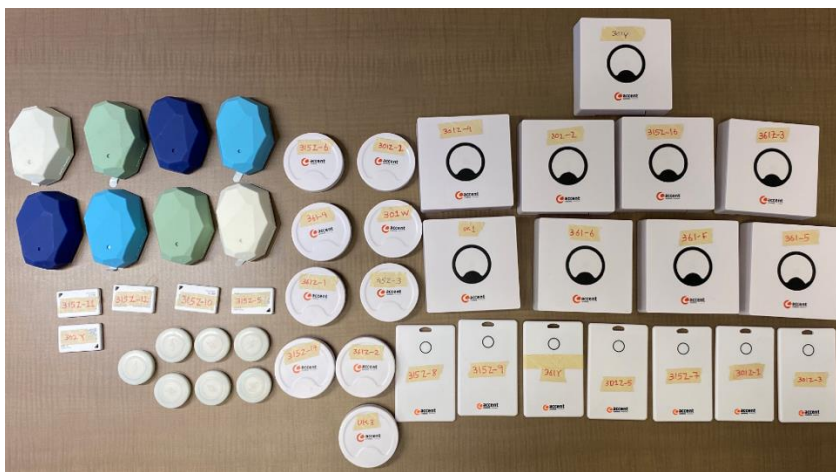
Figure 2.10. Six different types of BLE beacons from three different BLE manufacturers used in real-world experiment
