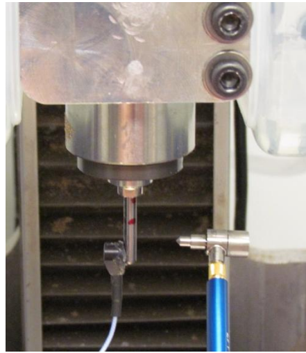
Figure 3.4 Hammer testing of blank end mill
