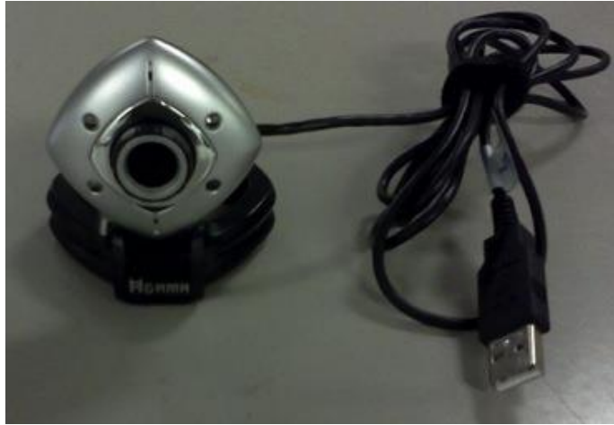
Figure 4.1: AGAMA V-1325R with a 2MP CMOS image sensor
