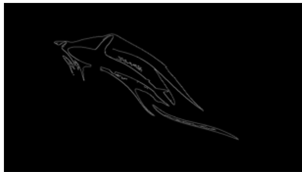
Figure 2.9b: Output after Canny edge detection
