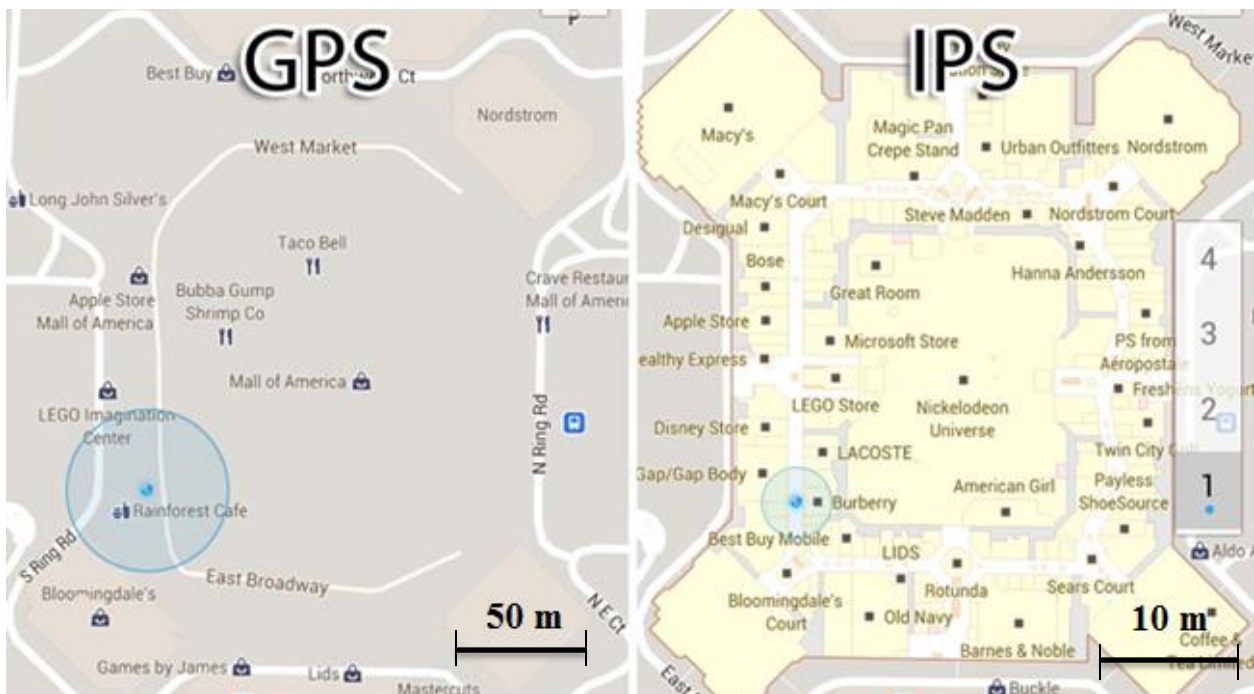
Figure 1.1: Difference in accuracy requirements between indoor and outdoor environments [6] Figure 1.1 illustrates the difference in the accuracy requirement between a global positioning system and an indoor positioning system (IPS). While the accuracy requirement for a GPS can
