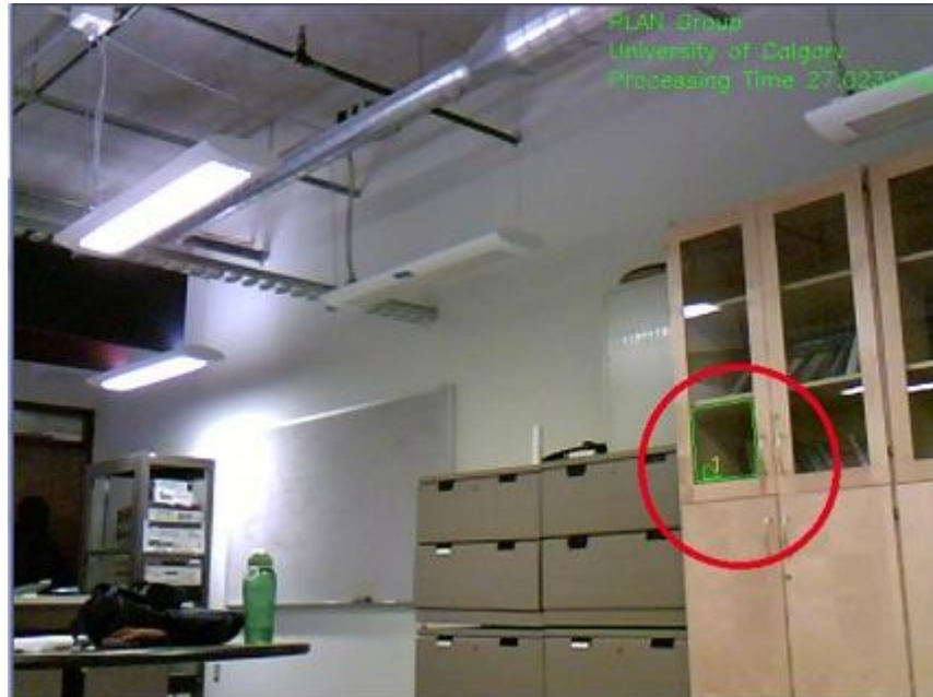
Figure 4.17: Detecting a cabinet window as a figure of opportunity
