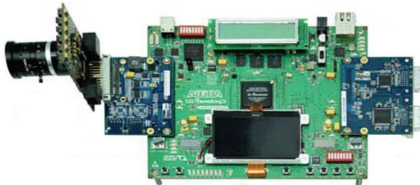
Figure 5-1 - Hardware system overview: WDR Image sensor on the left, development FPGA board in the middle and DVI PHY on the left
