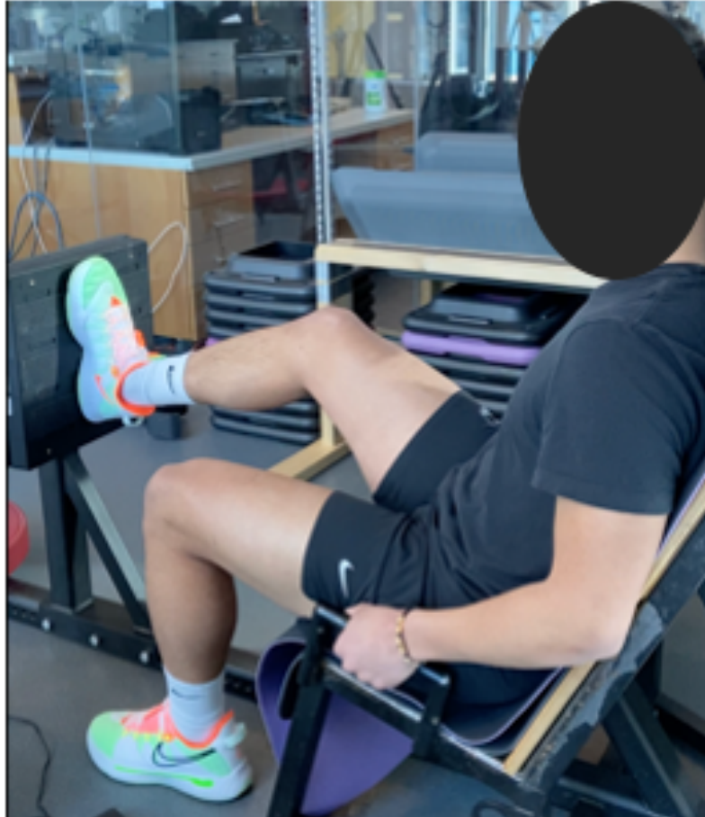
Figure 3.2 Isometric Leg Press Extension Testing Position. Subjects were seated at a hip angle of 100^{\circ} and knee angle at 60^{\circ} of knee flexion. The foot of the tested leg was centered on the vertically mounted force plate.
